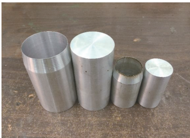
图 2 薄壁取心筒和取心圆柱 Fig. 2 Thin-wall coring cylinder and coring column
