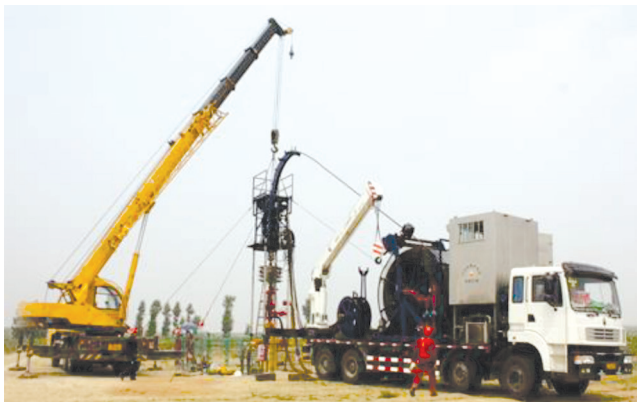
图4 长庆油田速度管柱排水采气施工现场图 Fig. 4 Working yard of unloading liquid using velocity string in Changqing oil field
